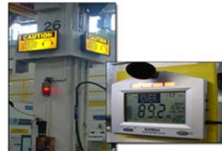
Noise is monitored throughout EHRO, with 14 meters connected to signs that light up when noise exceeds 82 dBA.
