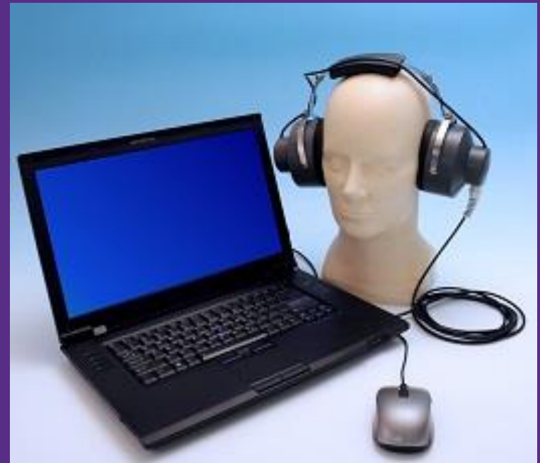
NIOSH HPD Well Fit™ fit testing system for earplugs. Photo by Mr. Scott Childress, US Army Aeromedical Laboratories
