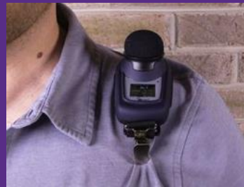
Sound Level Meter and Noise Dosimeter - OSHA Technical Manual
