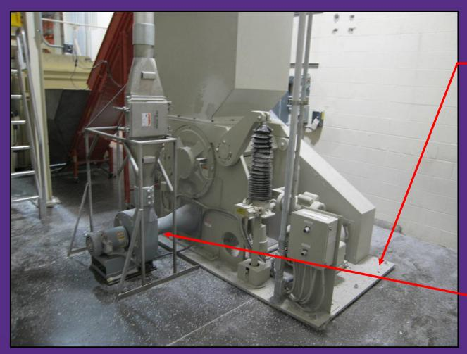
Dust build-up on floor around grinder due to inefficient regrind evacuation
