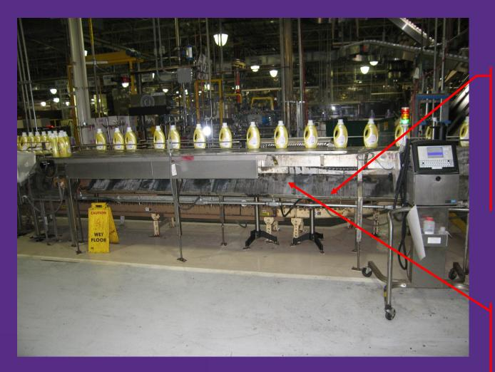
Line shaft removed; Individual drives installed: cleaner, quieter
