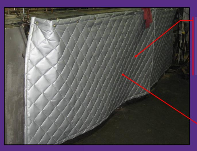
Even with sound barrier, motor, line shaft, and gearboxes were very loud
