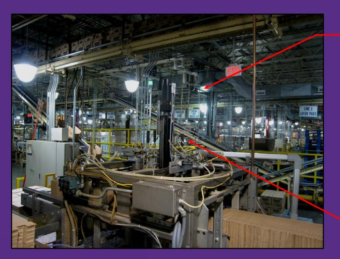
Conversion to servo-mandrel resulted in 72% reduction in air consumption, smoother stroke, less noise
