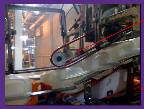
Replaced nozzles with in feed decline drive belt; reduced noise improved productivity
